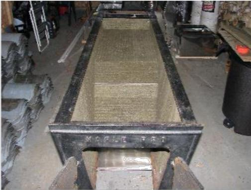
Insulating panels installed in the evaporator.
