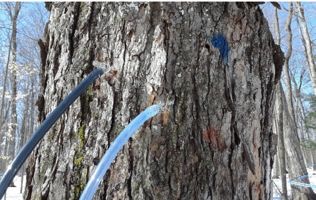
Fig. 1: Paired tapping system on the same trees, used to compare the blue (light) and grey (dark) tubing
