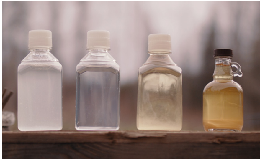
| From left to right: raw maple sap, ultrafiltered sap, ultrafiltered concentrated sap, 66 Brix maple nectar.
