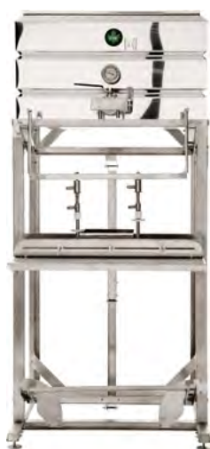
Electric water jacketed tank 43 US GAL. 67422
