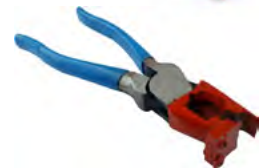
Stripping pliers Modified blade to facilitate cutting without breaking
