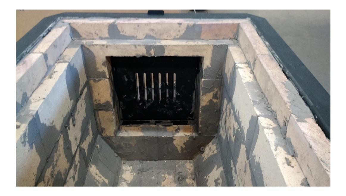
Leave to dry the cement during a minimum of 48 hours and then make a pre-cooking soft fire during 3 hours before use
