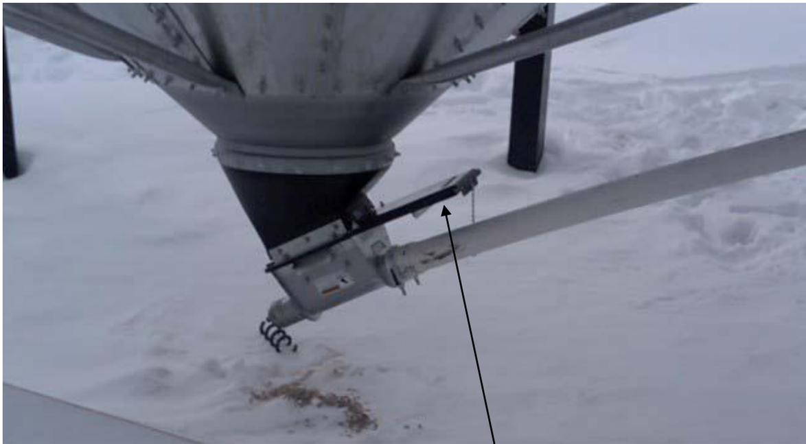
Silo gate valve, only open 1/3 in normal operation
