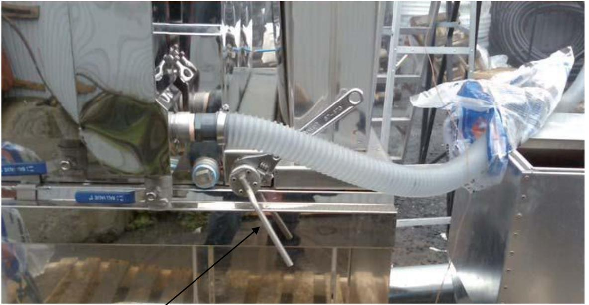
The damper will have to be adjusted between 35 to 45 degrés from the vertical. Magnehelic gauge must read 0.1.
