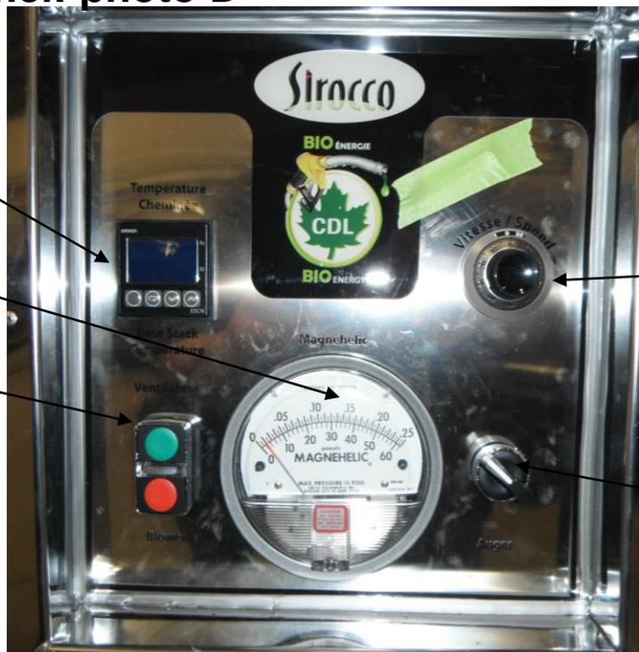
Pellet feed screw speed adjustment
