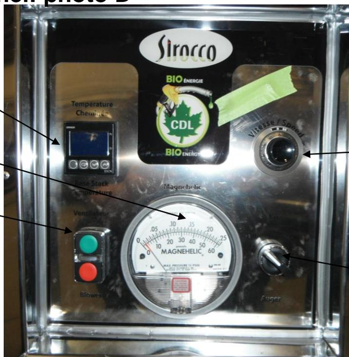
Pellet feed screw speed adjustment
