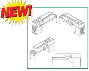
6700103 - 20" x 84" Wood Evaporator wth Dropped Flues SS Arch and 9" Stack List Price = \$4.930.00 2 - 20" x 15" SS Syrup Pans 20" x 54" SS Flue Pan (5" dropped flues) Front Float Boxes Large Level Gauge 24" Grates Hinged Stack Cover SS Draw-Off Valve
